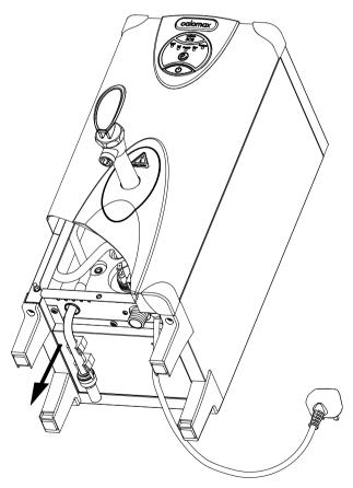
If the boiler is required to drip or overflow into the drip tray, the configuration of pipework may be altered as follows. Remove the machine front panel and unclip the pipework elbow. Carefully pull the elbow in the direction of the arrow, out of the silicone connecting tube on the end of the main water pipe. The silicone connecting tube will now direct water into the drip tray.
